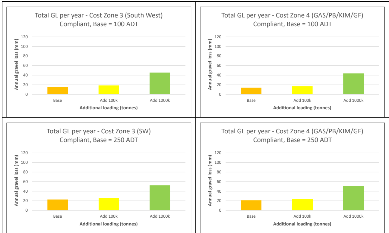
Figure 4.1 Annual gravel loss estimates for different base ADT and loading scenarios
